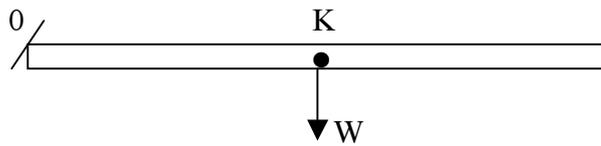
$$\left( \frac{dL}{dt} \right)_0 = \Sigma T(0) = T_{W(0)} = mg \frac{\ell}{2} = 15 \text{ Nm}$$
