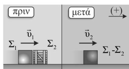
$$\text{A.Δ.O.: } \vec{p}_{\alpha\rho\gamma.\sigma\nu\sigma} = \vec{p}_{\tau\varepsilon\lambda.\sigma\nu\sigma} \quad \& \quad m_1 \cdot v_1 = (m_1 + m_2) \cdot v_2 \quad \& \quad v_2 = \frac{m_1 \cdot v_1}{m_2 + m_1} \quad \& \quad v_2 = 2 \text{ m/s}$$
